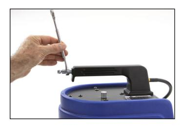
> If not supplied; install correct air fitting onto the Leakfinder®.
