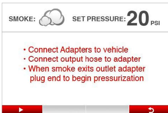
3. Follow on screen instructions and press the (
