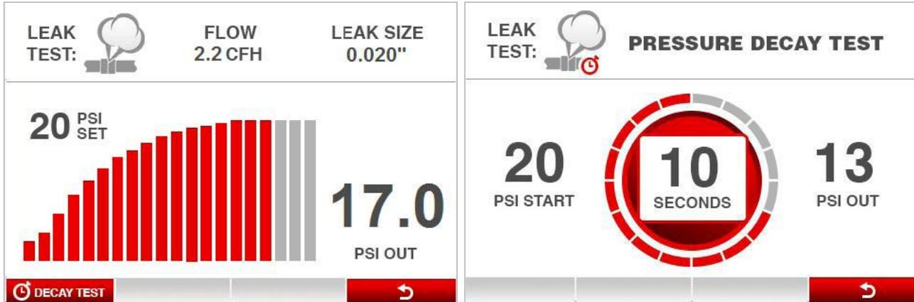
1. To perform a pressure decay test, begin a leak test. When the pressure has reached the set pressure. Press the “DECAY TEST” (
