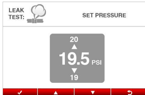
2. Set the test pressure by using the scroll buttons (
