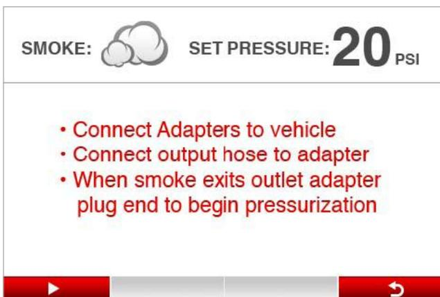
3. Follow on screen instructions and press the (
