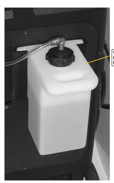
Waste (used) fluid capture tank The following safety instructions should be observed at all times when opening the MotorVac BRAKEVAC-II.
