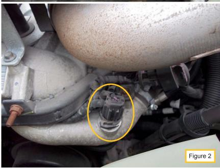
4. Remove EGR cooler temperature sensor (see figure 2). Disconnect EGR valve electrical connector to close the EGR valve (see figure 3 & 4).
