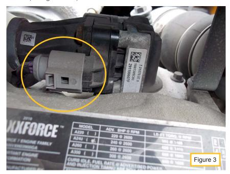
5. Install 069-3645 adapter (see figure 4) in place of above EGR temperature sensor.
