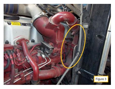
5. Install EGR adapter 069-3640 using the existing clamps. Tighten EGR cooler outlet pipe clamps (see figure 4).
