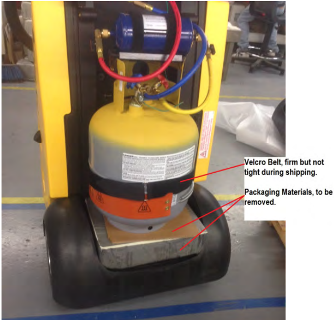
Figure A: Shipping support to be removed before start up.
