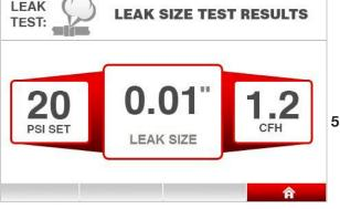
5. Results - When the output pressure stabilizes at the set pressure, the leak size results page will display the leak size and resulting flow rate from the test.
