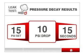
3. Results: When the pressure decay test is complete the results will be displayed. These results can be compared with the manufacturer's specifications.
