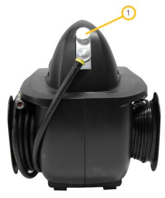
COOL SMOKE FLUID DIPSTICK: To check the fluid level insert dipstick until threads touch then remove and read. CAUTION: DO NOT OVERFILL THE UNIT.
