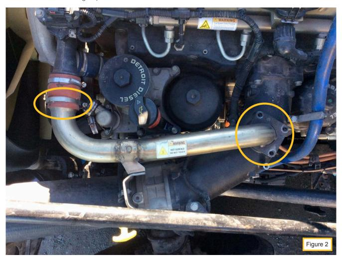
Quick Tip: Place the EGR cooler outlet pipe into a bucket/container and pour EGR fluid into the outlet pipe, this will aid in the dislodging of soot from the pipe while the EGR cleaning procedure is performed.
