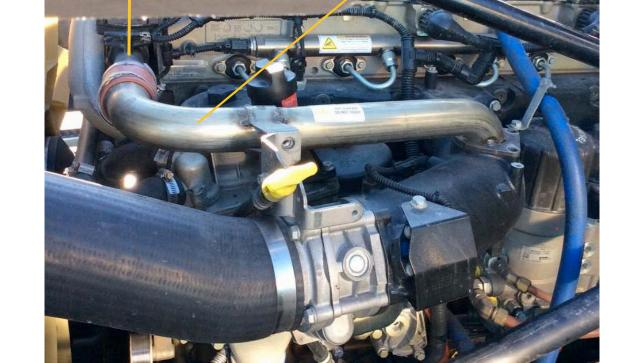
4. Remove the 3 bolts on the EGR cooler outlet (see Figure 2). Loosen the clamp on the rubber hose. Remove the EGR cooler outlet pipe and set it aside. The gasket on the EGR cooler outlet pipe will be used in the following steps.
