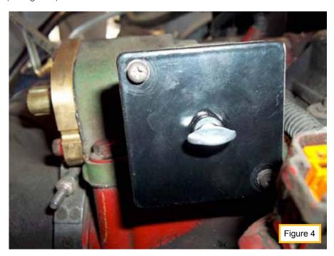
Note: For easier installation of 98821016 EGR manual valve opener, it is best to remove EGR valve assembly first (4 bolts). Install 98821016 and then reinstall EGR valve assembly.
