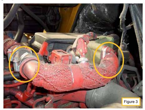
5. Turn thumbscrew on 98821016 fully counterclockwise but do not remove it from the adapter. Remove EGR valve solenoid (4 screws) and set aside, install 98821016 in its place using only two screws. Disconnect EGR valve solenoid electrical connector. Rotate thumb screw fully clockwise, EGR valve is now open (see figure 4).
