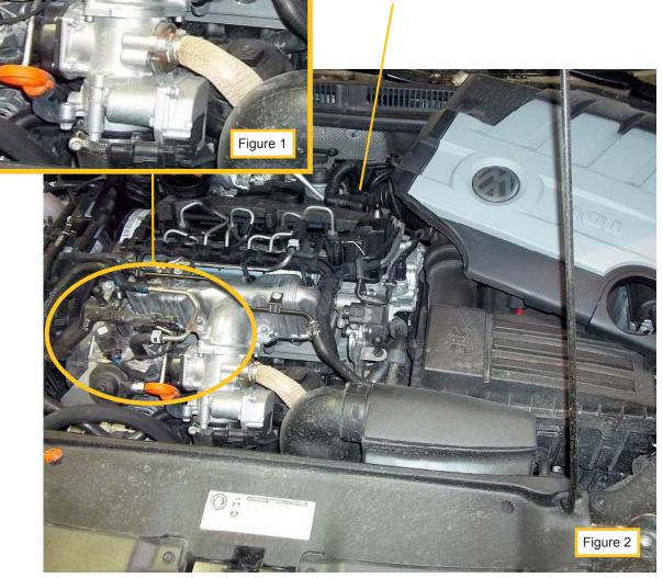
4. Remove EGR inlet pipe bolts (see figure 3). Pull back EGR pipe about ½" and remove gasket.
