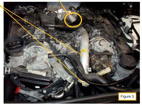
5. Remove EGR valve and set on top of engine with the electrical connector attached. Install 069-3519 in its place (see figure 4), install only 2 of the 3 bolts hand tight.
