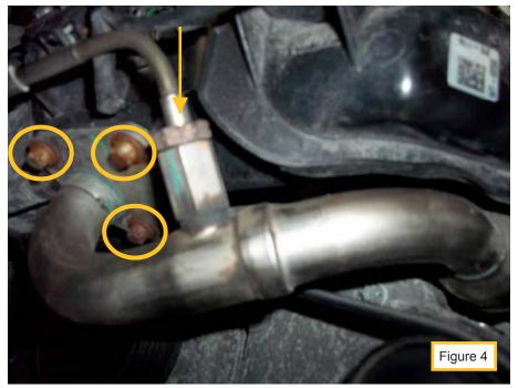
Quick Tip: Place the EGR cooler outlet pipe into a bucket/container and fill container with EGR fluid until submerged, this will aid in the dislodging of soot from the pipe while the EGR cleaning procedure is performed, see step 19.
