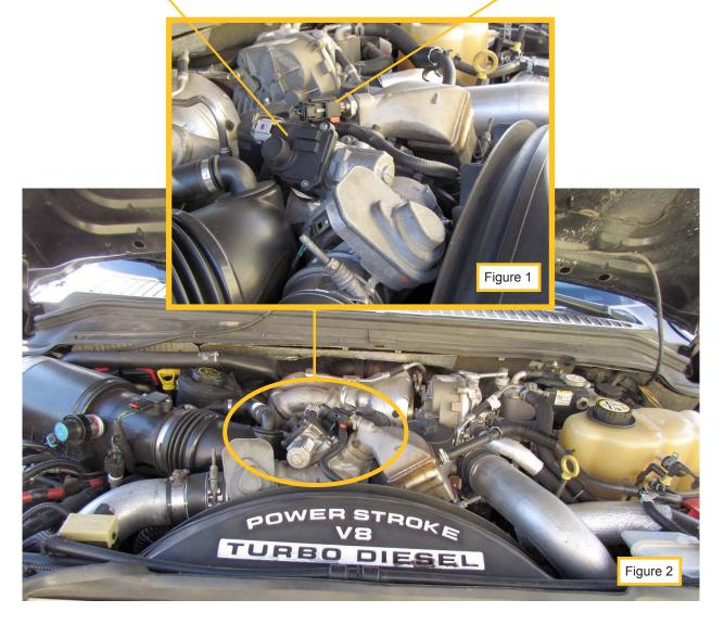
4. Remove EGR cooler temperature sensor (see figure 3). Disconnect EGR valve electrical connector to close the EGR valve.
